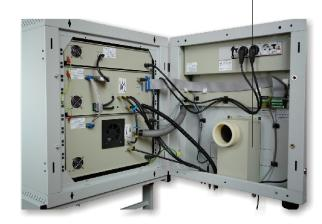
VIEW AT THE BACK PANELS OF ALL CMS-7 MODULES. CONNECTORS ARE ACCESSIBLE AFTER OPENING THE CABINET'S BACK DOOR.
